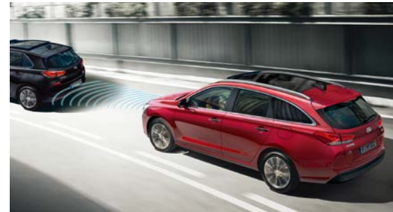
Advanced Smart Cruise Control (ASCC) maintains a pre-set distance to the preceding vehicle, automatically reducing or increasing speed as necessary.
