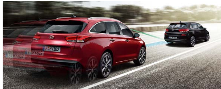
Autonomous Emergency Braking (AEB) with Pedestrian Alert function can apply partial or maximum braking force if a potential collision is detected.
